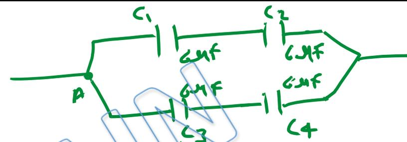
here  $C_1 = C_2 = C_3 = C_4 = C = 6\mu F$
