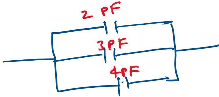
$$C_{eq} = C_1 + C_2 + C_3$$
