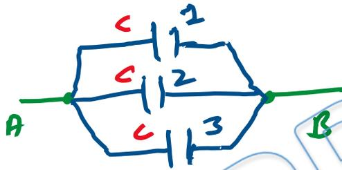
$$C_{eq} = C_1 + C_2 + C_3 \\ = C + C + C$$
